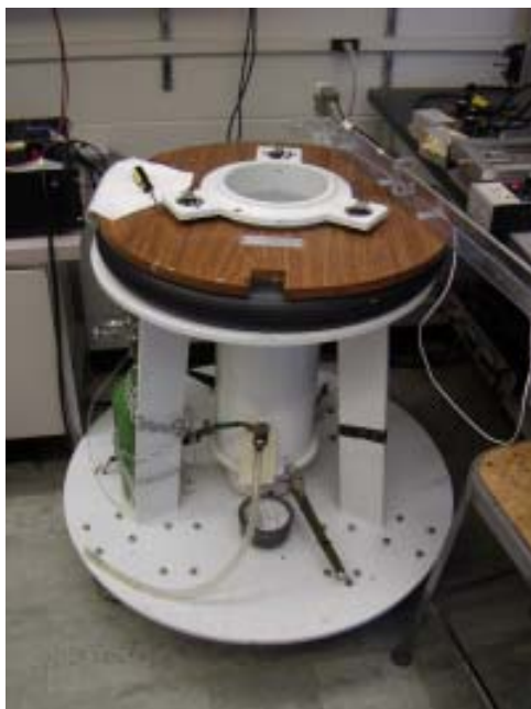
USRD type G40 calibrator used for the generation of low frequency underwater sound fields in the 100 - 1000 Hz range.
