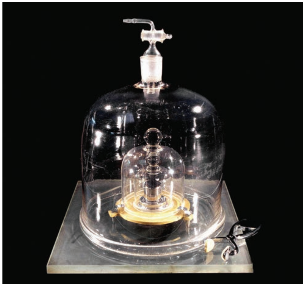
SAFE KEEPING: “Le Grand K,” the original platinum and iridium cylinder that is still the international prototype for the kilogram weight, sits under three bell jars in the suburbs of Paris.
