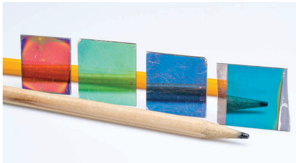
BOTH SIDES NOW: Rochester-developed coatings simultaneously reflect and transmit the same wavelength.
